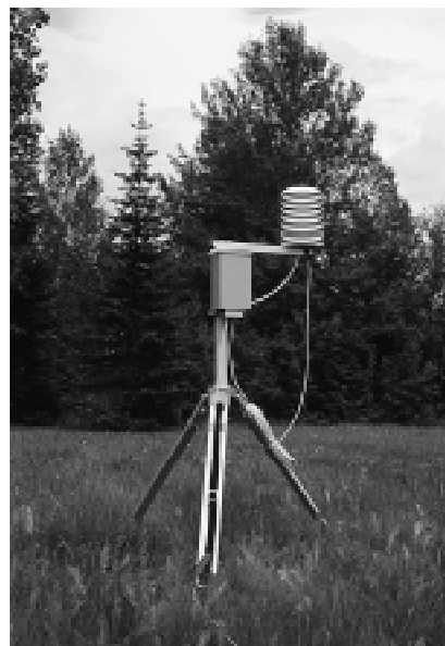
PTU 200 shown with meteorological installation kit (PTU 200 MIK) and tripod.
